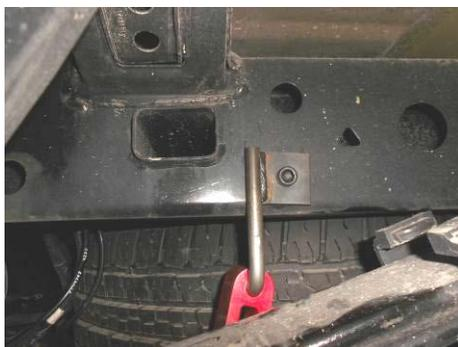
1) Mount the left rear tailpipe hanger bracket **#226HA** to the frame on the driver's side of the vehicle. Place the included 3/8 x 3.50" bolt thru the 226HA hanger and into the hole indicated in the photo. On the inside of the frame, place the HA226 back-up plate over the bolt followed by a flat washer, lock washer and nut. Using two 9/16" wrenches tighten firmly (Do not over tighten).
