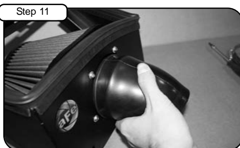
Step 11 Attach the coupler with the clamps provided to the filter adaptor. Do not tighten clamps.
