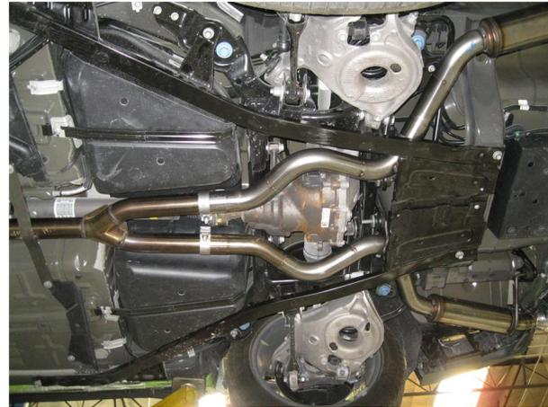
**Step 3.** Next attach the Extension Pipe Assemblies to the Y-Pipe using the supplied 2.50" clamps and fitting the hangers into the rubber insulators.
