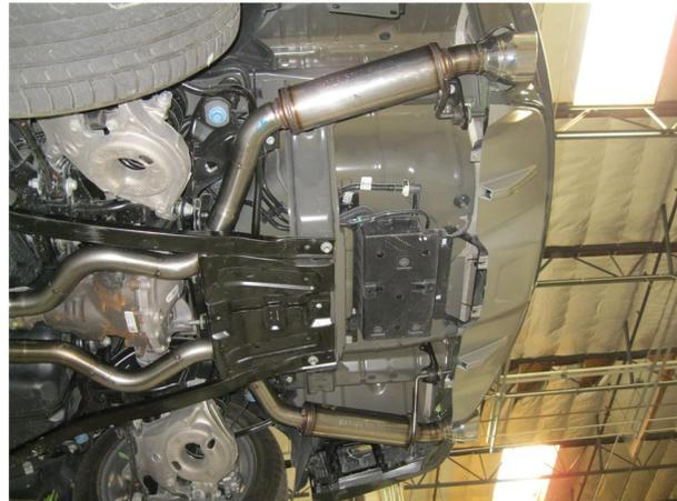
**Step 4.** Finish the initial installation by fitting the Muffler Assemblies onto the Extension pipes using the supplied 3.00" clamps and inserting the hangers into the rubber insulators.
