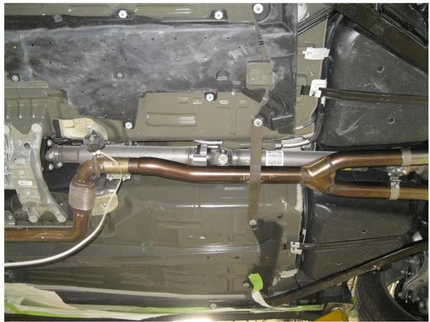
**Step 2.** Begin installation of the new system by loosely attaching the Y-Pipe Assembly to the outlets using the OEM clamp. Leave all clamps loose until final adjustment.
